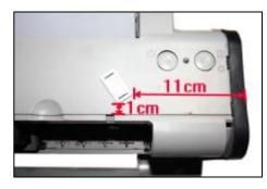
Fix the supporting arm as the picture shows. Measure 11 cm from the right edge of printer, 1 cm from the below edge, which forms an angle of 60°.
